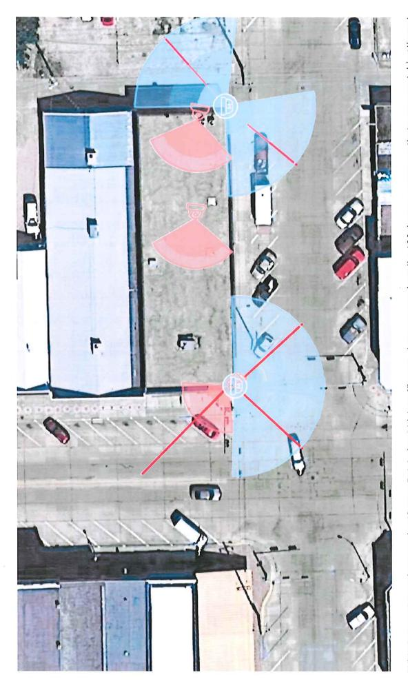
With that southwest intersection/Corner Pub being a high traffic area, I propose we install a 180 degree camera on that corner watching these t would then install a camera under the awning (in red), watching the sidewalk/entrance/street parking.
